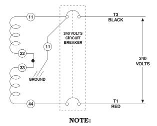
Do NOT connect loads in excess of circuit breaker ratings.
